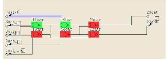
Figure 5: Using the expanded node model, gate 23GAT could have its input shorted to ground. Causing a symptom at 22gat (should be 0 but 1 is measured). The likely faulted gates are now 10GAT, 16GAT, 22GAT and 23GAT.
